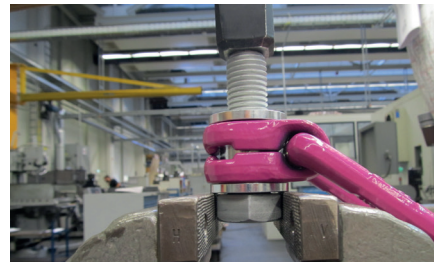
Pic. 8: Dismantling position of the VLBG
