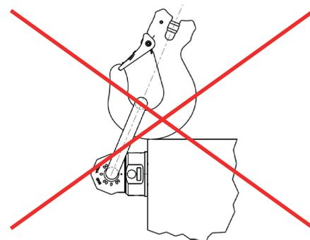
Fig. 2: Forbidden contact and/or support on edges
