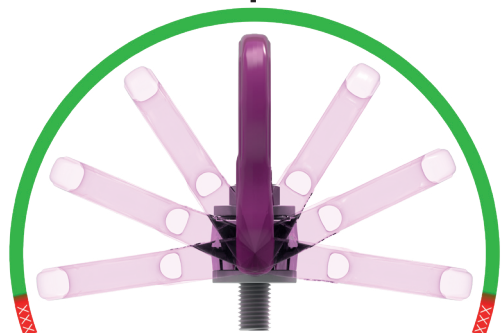
Pic. 11: Pivoting area (green = permitted loading direction)
