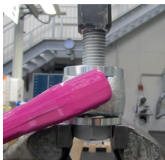
Pic. 12: Supporting position of the ACP on of the vice jaws
