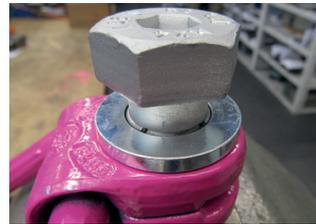
Pic. 7: Retaining ring positioned as circumferential in the recess
