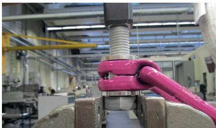
Pic. 5: Dismantling position of the L-VLBG
